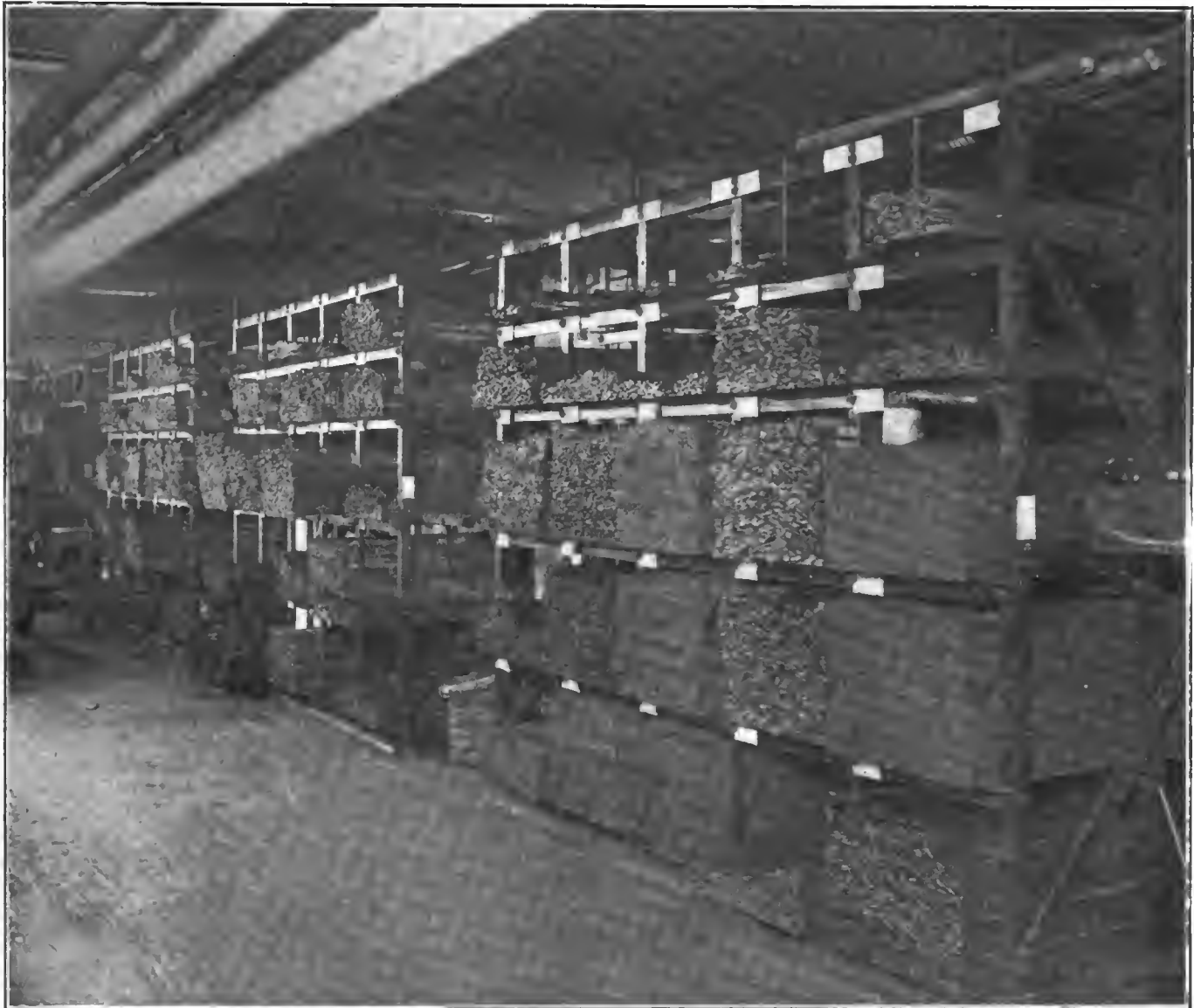
GOOD MATERIALS MUST BE CAREFULLY STORED AND PREVENTED FROM BEING MIXED—DIAMOND CHAIN METHOD
